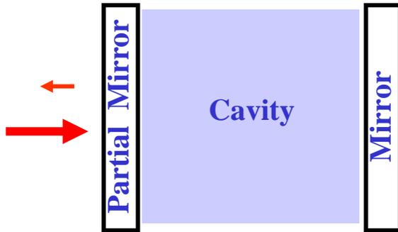
Uniform resonance cavity with photonic reflectors (DBR)
