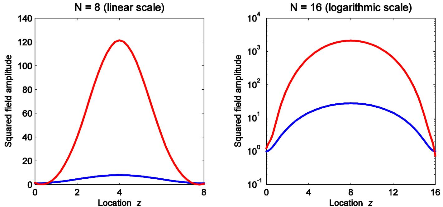
Energy density distribution inside photonic crystal at frequency of slow wave resonance
