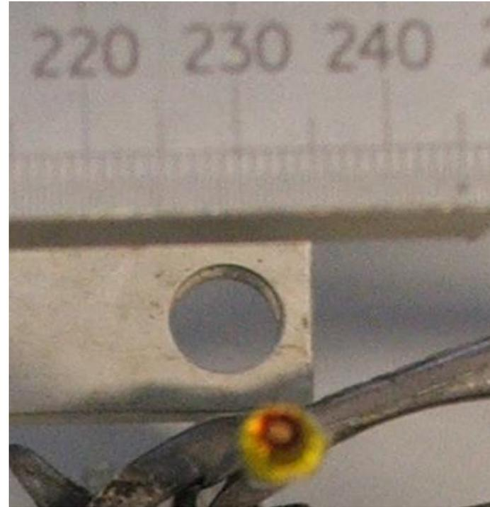
Beam profile displayed as red ring on electron sensitive film
