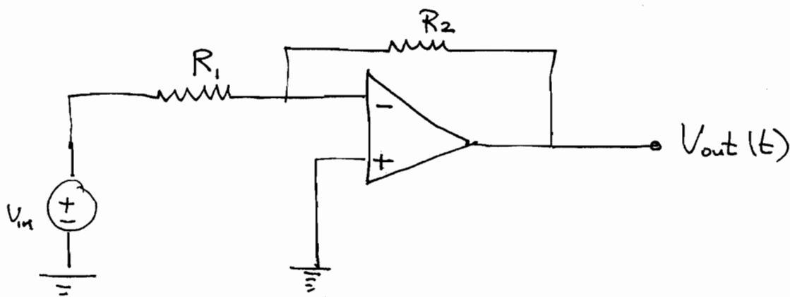
$$\frac{V_{out}(j\omega)}{R_2} - \cancel{V_-}^o + \frac{V_{in}(j\omega) - \cancel{V_-}^o}{R_1} = 0$$
