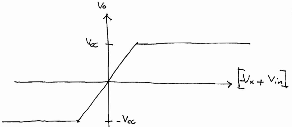
Linear Region  $|V_x - V_{in}| < \frac{V_{cc}}{A}$
