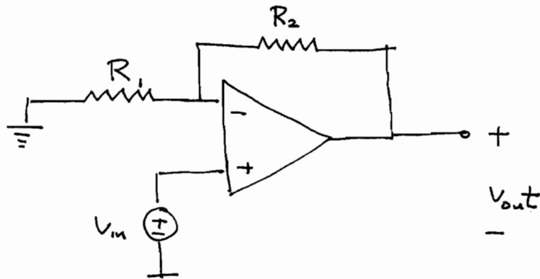
$$\frac{V_{out}(j\omega)}{R_2} - \cancel{V_-} + \frac{0 - \cancel{V_-}}{R_1} = 0$$
