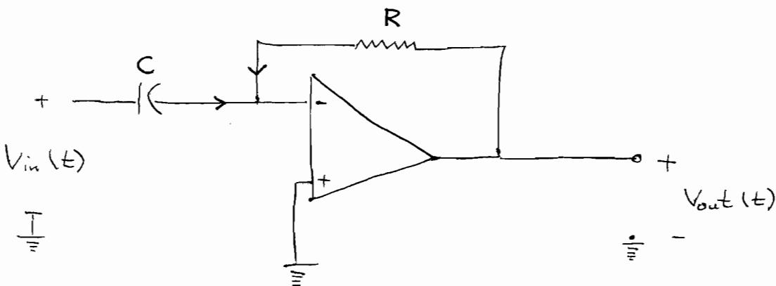
$$\frac{V_{out} - V_-}{R} + \frac{V_{in} - V_-}{\frac{1}{j\omega C}} = 0$$
