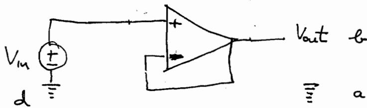
$$V_o = V_- = V_+ = V_{out}$$
