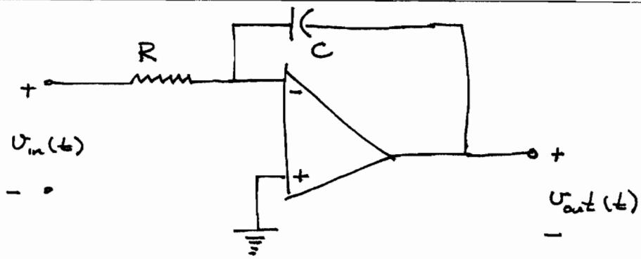
$$\frac{V_{out}(j\omega) - V_-}{\frac{1}{j\omega C}} + \frac{V_{in}(j\omega) - V_-}{R} = 0$$
