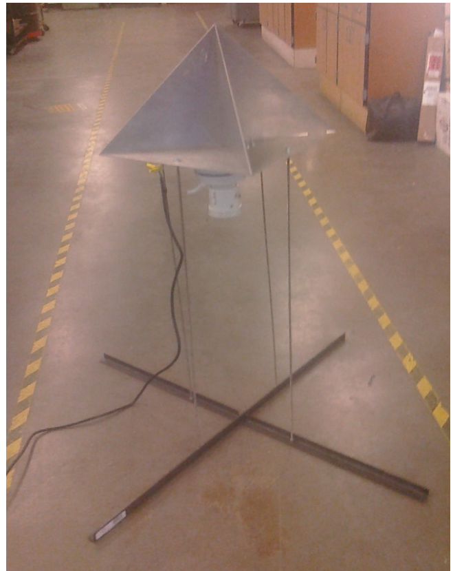
Fig. 5: Vibrating target in a machine shop. It is an aluminum triangular trihedral with lateral length of 12 inches and it vibrates at 7 Hz with an amplitude of 0.5 mm.
