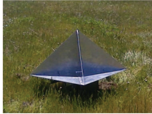
Fig. 1. Vibrating retro-reflector on the test ground near Julian, CA. The target is an aluminum triangular trihedral with lateral length of 21 inches. The vibration frequency and amplitude were 0.8 Hz and 1.5 cm, respectively.
