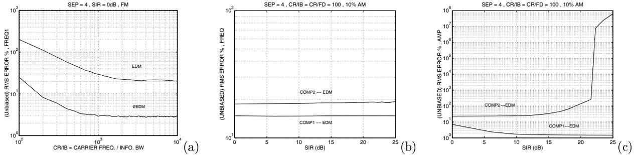
Fig. 2. (a) Effect of CR/IB on EDM frequency demodulation obtained by averaging over FM modulation indices  $\in \{0.1 - 1\}\%$ . (b,c) Effect of SIR on EDM frequency and amplitude demodulation.
