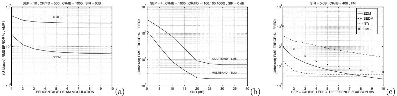
Fig. 3. (a) Comparison of amplitude demodulation between the SEDM and the SITD for different AM modulation percentages. (b) Effect of SNR on the performance of the multiband-EDM (MEDM) and the multiband-LMS (MLMS) (averaged over various CR/FD). (c) Effect of spectral separation on the performance of the EDM, the ITD and the LMS (averaged over CR/FD).
