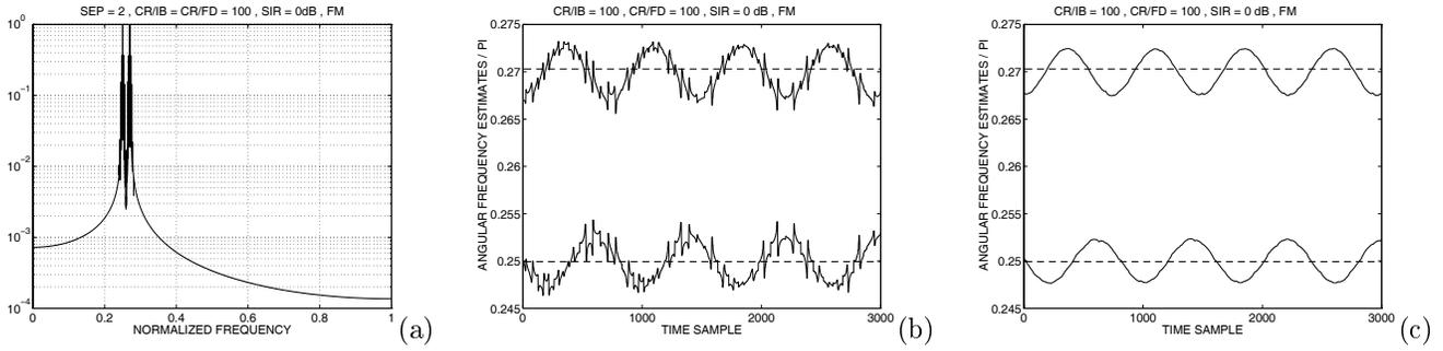
Fig. 1. (a) Fourier spectral magnitude of mixture signal. (b) Angular frequency estimates of the EDM as fractions of  $\pi$ . (c) Frequency estimates of the SEDM, i.e. the estimates in (b) after post-smoothing.
