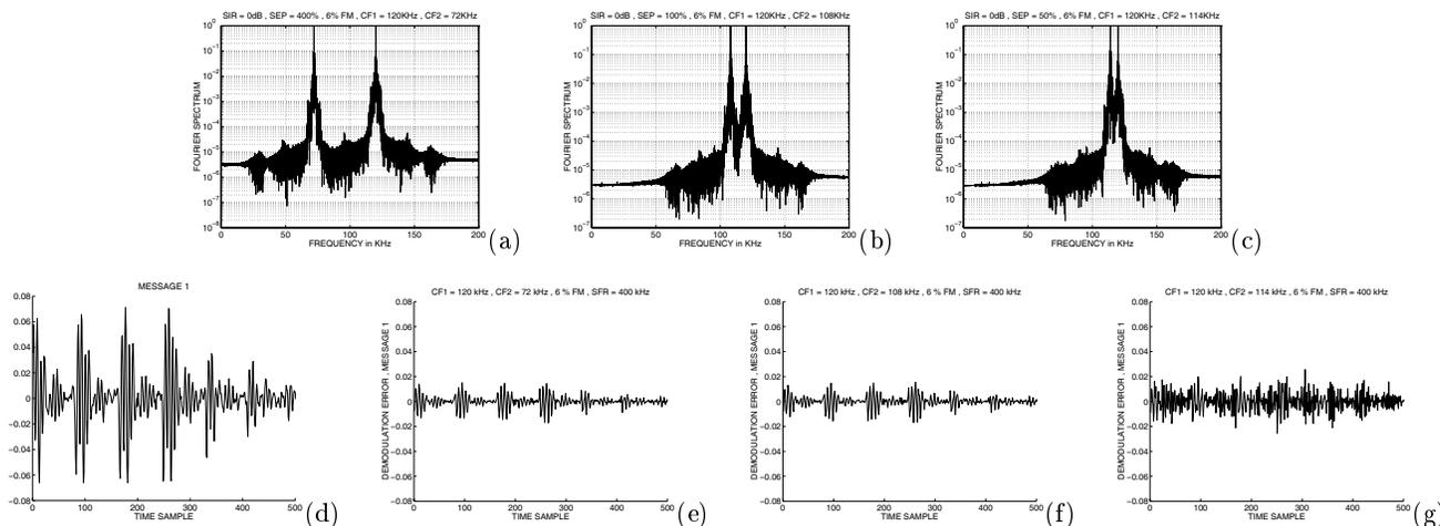
Figure 2. (a,b,c) are the spectra of the composite signal for normalized carrier separations of {400, 100, 50}%. (d,e,f,g) are the original voice signal and the demodulation errors for the first signal component at normalized carrier separations of {400, 100, 50}%, pertaining to the EDM-related voice experiments.
