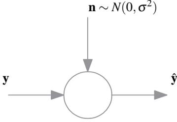
Fig. 5 AWGN channel scheme.
