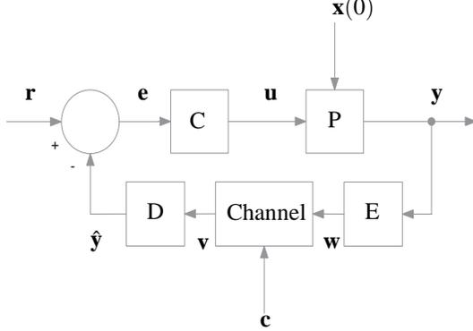
Fig. 1 Closed-loop system with communication channel in feedback Link.
