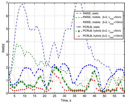
Fig. 4. RMSE and PCRLB (in  $m$ ) for the estimated target position when  $v_{max}$  is varying;  $n_s = 36$ ,  $n_m = 12$ ,  $C = 4$ ,  $v_{min} = 0$ ,  $r_D = 5m$ ,  $\beta = 2$
