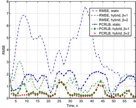
Fig. 3. RMSE and PCRLB (in  $m$ ) for the estimated target position when  $\beta$  is changing;  $n_s = 36$ ,  $n_m = 12$ ,  $C = 4$ ,  $v_{max} = 10ms^{-1}$ ,  $v_{min} = 0$ ,  $r_D = 5m$
