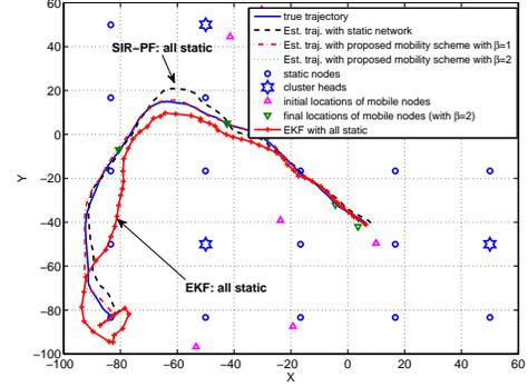
Fig. 2. Estimated trace of the target trajectory with proposed MAT algorithm;  $n_s = 36$ ,  $n_m = 12$ ,  $C = 4$ ,  $v_{max} = 10ms^{-1}$ ,  $r_D = 5m$
