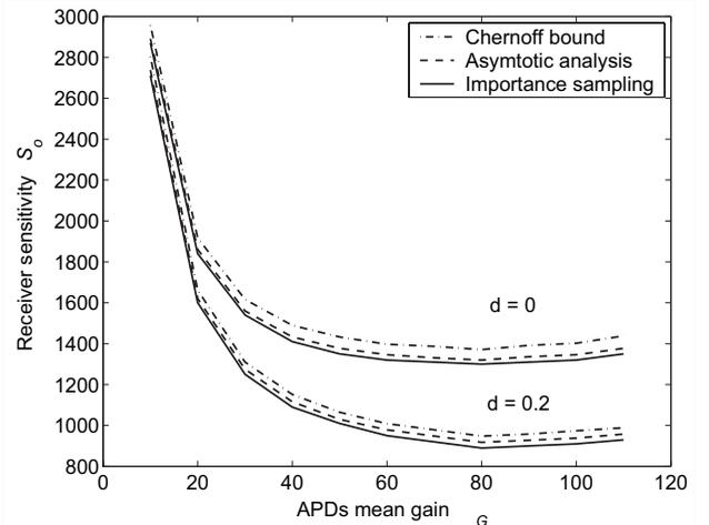
Fig. 2: Receiver sensitivity as a function the APD's mean gain  $\mu_G$  for  $d = 0$  and  $d = 0.2$ . It is assumed that  $\sigma^2 = 8 \times 10^6$  and that each incident photon results in a primary electron.
