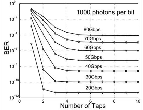
Fig. 2: BER of the receiver with the RD-model equalizer as a function of the number of taps,  $M$ , for various level of input optical signal intensity.
