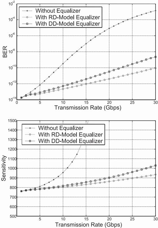
Fig. 1: BER and receiver sensitivity as a function of the transmission rate.
