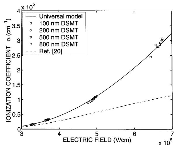
Fig. 2. Electron ionization coefficient ( $\alpha$ ) of GaAs as a function of the electric field. Symbols represent the ionization coefficients of enabled carriers obtained from the data of four thin GaAs APD's [16] in conjunction with the DSMT while the solid curve represents the universal exponential model for these coefficients. The dashed curve represents the effective ionization coefficients obtained by [20] using the McIntyre theory [3] on bulk GaAs.
