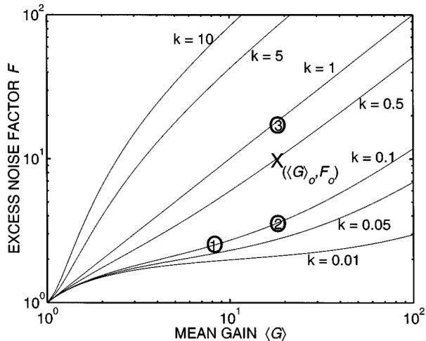
Fig. 1. Excess noise factor ( $F$ ) versus mean gain ( $\langle G \rangle$ ) characteristics of an APD parameterized by the ratio of the hole coefficient to electron coefficient  $k$ , according to the conventional McIntyre theory [3]. The points 1, 2, and 3 illustrate samples of  $(\langle G \rangle, F)$  pairs generated in the process of finding the ionization coefficients of enabled carriers using the dead-space theory.
