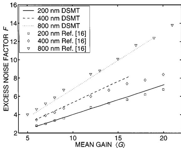
Fig. 7. Comparison of the DSMT-predicted and experimental excess noise factor  $F$  and mean gain  $\langle G \rangle$  for three thin  $\text{Al}_{0.2}\text{Ga}_{0.8}\text{As}$  APD's with different multiplication-region widths. Plot symbols are the same as in Fig. 6.
