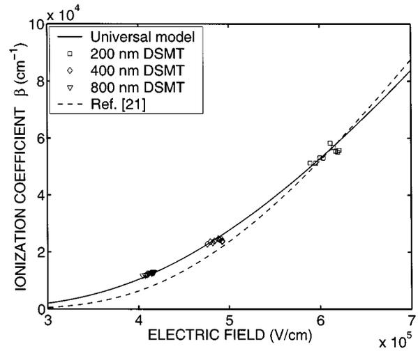
Fig. 5. Hole ionization coefficient ( $\beta$ ) of  $\text{Al}_{0.2}\text{Ga}_{0.8}\text{As}$  as a function of the electric field. Plot symbols are the same as in Fig. 4.
