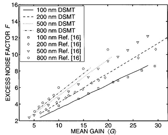
Fig. 6. Comparison of the DSMT-predicted and experimental excess noise factor  $F$  and mean gain  $\langle G \rangle$  for four thin GaAs APD's with different multiplication-region widths. Symbols represent experimental data (obtained from [16]) and curves represent the predictions using the DSMT.
