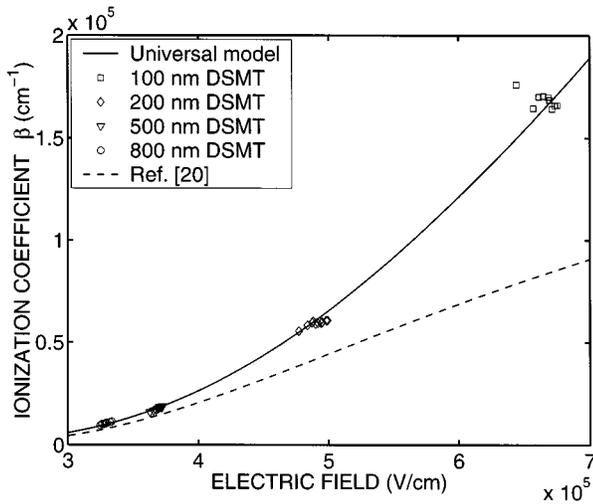
Fig. 3. Hole ionization coefficient ( $\beta$ ) of GaAs as a function of the electric field. Plot symbols are the same as in Fig. 2.
