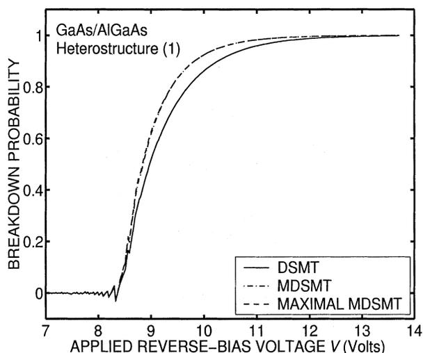
Fig. 5. Breakdown probability versus applied reverse-bias voltage for the first heterostructure GaAs–Al<sub>0.6</sub>Ga<sub>0.4</sub>As APD, which has a GaAs multiplication-region width of 130 nm. Three separate curves are shown representing the DSMT-predictions (solid), the MDSMT predictions (dotted-dashed), and the maximal-MDSMT predictions (dashed).
