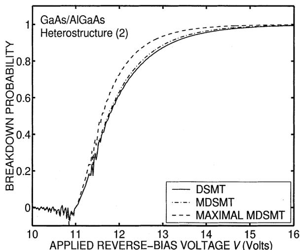
Fig. 6. Same as Fig. 5 but for the second GaAs–Al<sub>0.6</sub>Ga<sub>0.4</sub>As heterostructure, which has a two-layer Al<sub>0.6</sub>Ga<sub>0.4</sub>As–GaAs multiplication region width total width of 130 nm.
