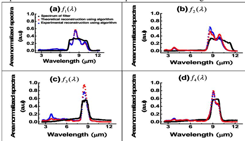
**Fig. 1.** Experimental results: constructions of four LWIR test filters obtained using the bias dependent photocurrent from a multi stack quantum dots in a well (DWELL) detector. Black: the true spectra of 4 LWIR filters; red: the theoretical estimations using algorithm; blue: the experimental reconstructions using algorithm without physical spectrometer.
