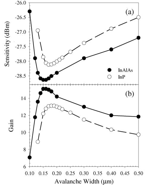
Fig. 1. (a) Optimum sensitivity and (b) the corresponding mean gain versus device avalanche width for a 10-Gb/s system using InAlAs (closed symbols) and InP (open symbols) APDs. Lines are drawn to aid visualization.
