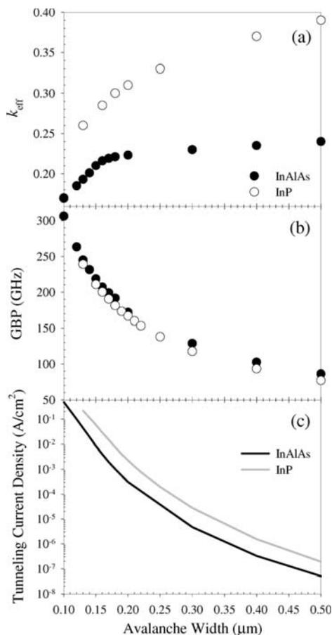
Fig. 2. (a) Effective ionization coefficient ratio ( $k_{eff}$ ), (b) gain-bandwidth product, and (c) tunneling current density, all functions of the avalanche width for a 10-Gb/s transmission system using InAlAs (closed symbols; black line) and InP (open symbols; gray line).
