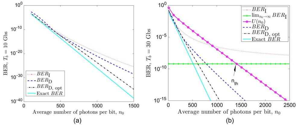
Fig. 2. The BER of an InP-based optical receiver using the two approximation methods compared to the exact BER. In the PD method, the optimal threshold,  $\theta_o$ , was considered in addition to the suboptimal threshold,  $\theta$  ( $L = 5$ ). (a) BER at a transmission rate of 10 Gb/s. (b) BER at a transmission rate of 30 Gb/s.
