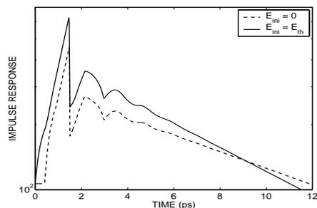
Figure 2. Mean impulse response of a 100-nm homojunction GaAs APD with no initial energy ( $E_{ini} = 0$ , dashed curve) and with maximal initial energy ( $E_{ini} = E_{th} = 1.9$  eV, solid curve).
