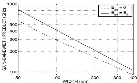
Figure 3. GBP of a 100-nm homojunction GaAs APD showing the effect of the absence (dashed curve) and presence (solid curve) of the initial energy.
