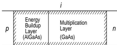
Figure 1. Schematic of a heterostructure APD which is used exploit the bandgap-boundary effect.
