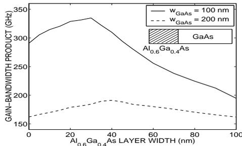
Figure 4. Dependence of the gain-bandwidth product in a heterostructure APD on the width of the  $\text{Al}_{0.6}\text{Ga}_{0.4}\text{As}$  energy-buildup layer.
