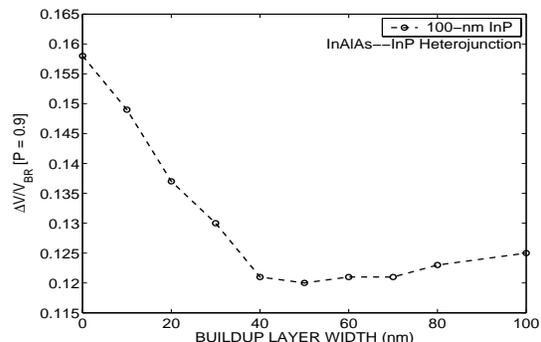
Figure 2. Normalized excess voltage when the breakdown probability is 0.9 as a function of  $\text{In}_{0.52}\text{Al}_{0.48}\text{As}$ -buildup-layer width.
