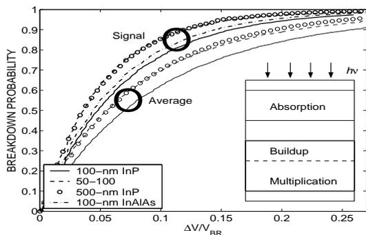
Figure 1. Breakdown probability as a function of normalized excess voltage ( $\Delta V/V_{BR}$ ). The inset depicts the schematic of the proposed structure.
