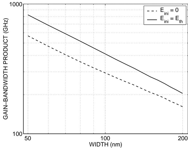
**Figure 6.** Gain-bandwidth product as a function of the width of the multiplication region for GaAs APDs. The top curve assumes maximal initial energy, equal to the ionization threshold energy, and the bottom curve assumes zero initial energy.
