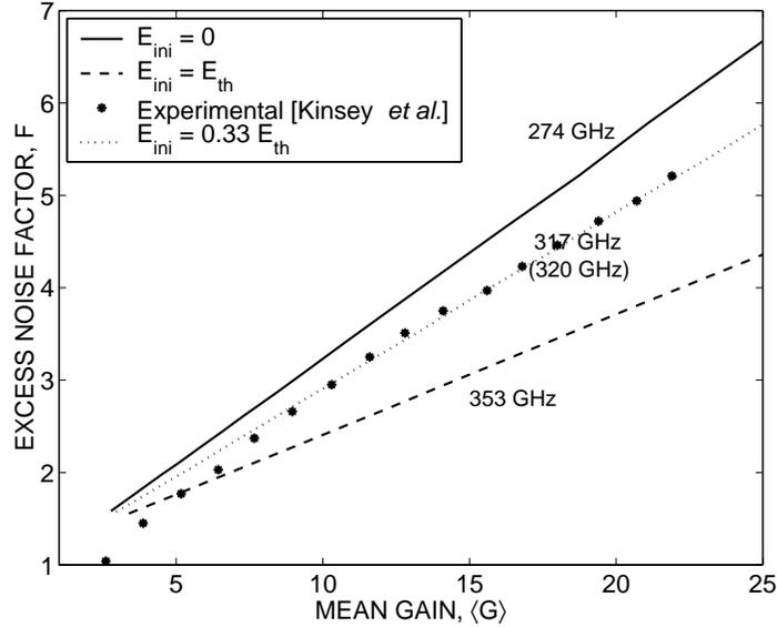
**Figure 7.** Excess noise factor as a function of the mean gain for a waveguide InAlAs APD developed by Kinsey *et al.*<sup>2,5</sup> The case  $E_{ini} = 0.33E_{th}$  yields the best noise-gain fit to data. The calculated GBP for this case is 317 GHz, which is in close agreement with the measured GBP of 320 GHz. The cases of  $E_{ini} = 0$  and  $E_{ini} = E_{th}$ , respectively, yield theoretical GBPs of 353 GHz and 274 GHz.
