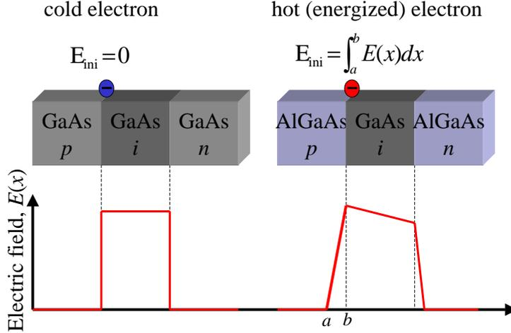
**Figure 1.** The device on the left does not exhibit the initial-energy effect since electrons are injected into the  $i$  multiplication layer without substantial energy (cold-electron injection). The device on the right exhibits a narrow high-field region (from  $a$  to  $b$ ) where electrons can build up a substantial energy  $E_{ini}$  prior to entering the  $i$  layer. The electrons are therefore injected hot in the latter case.
