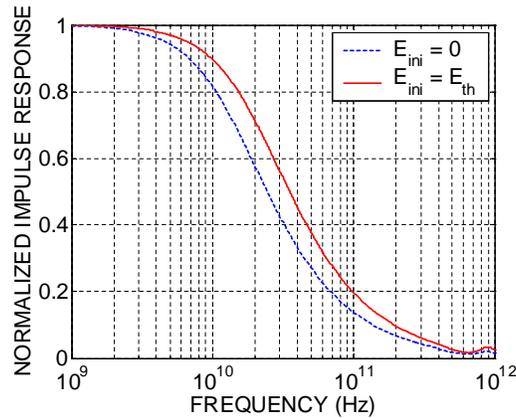
**Figure 5.** The calculated frequency response of a GaAs APD with a 100-nm multiplication region showing the bandwidth enhancement due to the initial-energy effect. The solid curve (top) represents the case when the initial energy of injected carriers is equal to the ionization energy and the dashed curve (bottom) corresponds to the case where zero-initial energy is present. The mean gain in both cases is 10.
