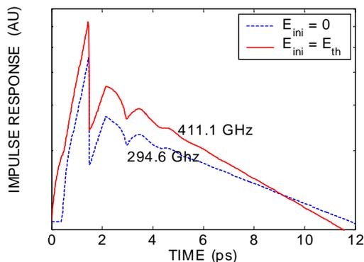
**Figure 4.** The calculated mean impulse response function of a GaAs APD with a 100-nm multiplication region. The solid curve represents the case when the initial energy of injected carriers is equal to the ionization energy and the dashed curve corresponds to the case where zero-initial energy is present. The mean gain in both cases is 10.
