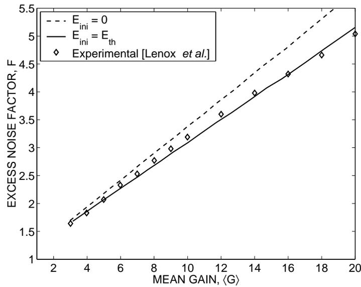
**Figure 3.** The calculated excess noise factor, as a function of the mean multiplication (gain), for an InAlAs APD with a 200-nm multiplication layer. The calculations are parameterized by the initial energy for two cases:  $E_{ini} = 0$  and  $E_{ini} = E_{th}$ . The case  $E_{ini} = E_{th}$  produces the best match with the experimental results (symbols) reported by Lenox *et al.*<sup>3</sup>
