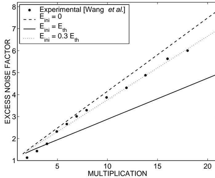
**Figure 2.** The calculated excess noise factor, as a function of the mean multiplication (gain), for a GaAs APD with a 153-nm multiplication layer. The calculations are parameterized by the initial energy for three cases:  $E_{ini} = 0$ ,  $E_{ini} = 0.3E_{th}$ , and  $E_{ini} = E_{th}$ . The case  $E_{ini} = 0.3E_{th}$  produces the best match with the experimental results (symbols) reported by Wang *et al.*<sup>28</sup>
