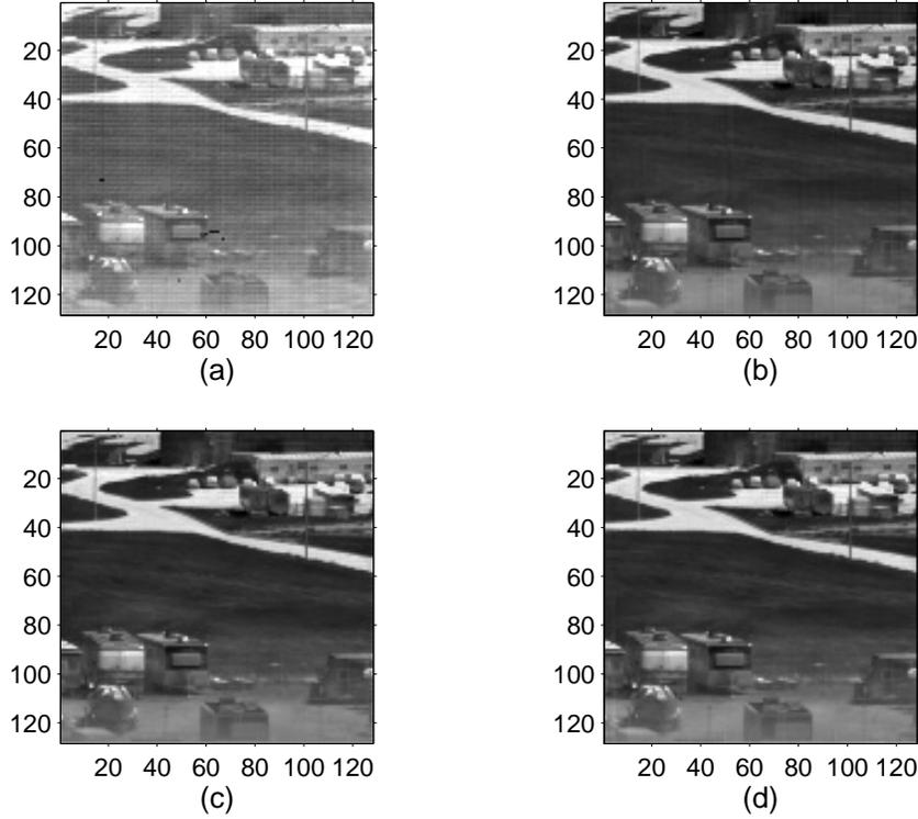
**Figure 5.** Image frame 325 from Data Set 1: (a) Raw image; (b) After correction by the ASBA; (c) After correction by the RASBA; (d) After correction by the GASBA. All images are statistically scaled to the same dynamic range.
