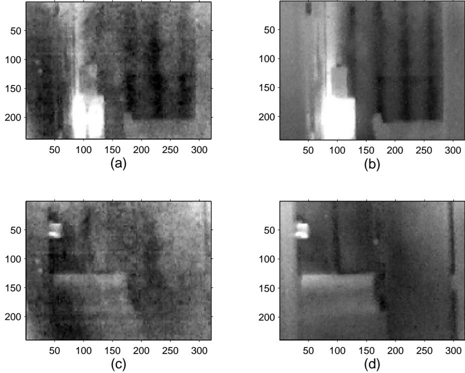
**Figure 6.** Imagery from Data Set 2: (a) Raw image frame 1750; (b) Image frame 1750 after correction by the GASBA. Imagery from Data Set 3: (c) Raw image frame 480; (d) Image frame 480 after correction by the GASBA. All images are statistically scaled to the same dynamic range.
