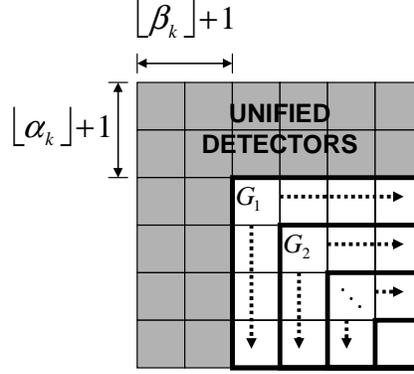
**Figure 3.** Graphical representation of the recursive operation of the algorithm. The unshaded pixel partitions correspond to each  $G_\ell$ , representing the group of detectors whose biases are estimated iteratively in  $\ell$ . The arrows indicate the direction of algorithm iteration within each  $G_\ell$ .
