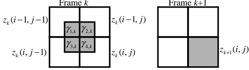
**Figure 1.** Graphical depiction of the bilinear irradiance interpolation model for the case of subpixel 2D motion. The pixels shaded in blue represent the interpolated IR-signal value at time  $k + 1$ .
