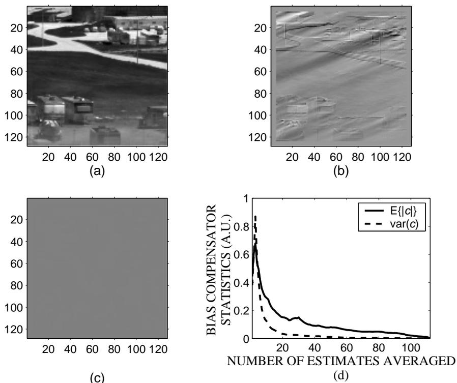
**Figure 8.** (a) Image frame 500 from Data Set 1 after correction by the GASBA; (b) Bias compensator estimates produced from the correction of frames 500 and 501 (linearly scaled to the full dynamic range); (c) Bias compensator estimates after averaging 116 estimate matrices; (d) Plot showing the mean and variance of the bias compensator estimates as a function of the number of estimates in the average.
