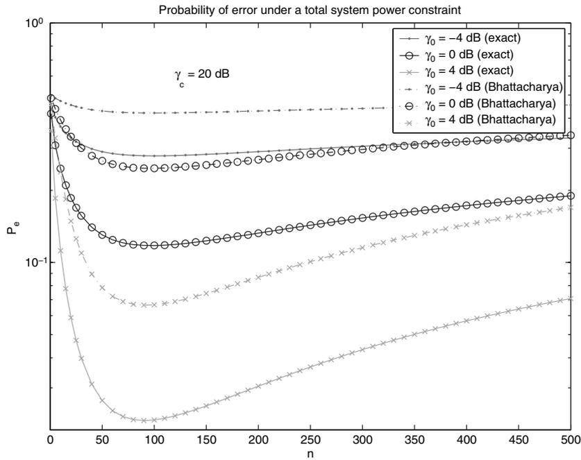
Figure 6.5 Exact and the Bhattacharyya Upper-bound to the Minimum Achievable Fusion Probability of Error in Distributed Detection of a Random Signal with Orthogonal Sensor-to-Fusion Center Communication under a Global Power Constraint.  $\gamma_c = 20$  dB
