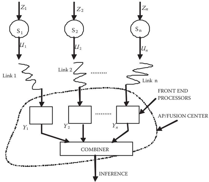
Figure 6.1 Parallel Data Fusion Model in Sensor Network
