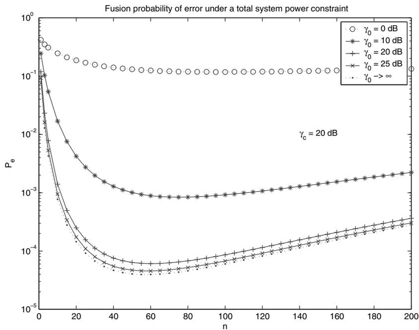
Figure 6.6 Large  $\gamma_0$  Limiting Behavior of the Minimum Achievable Fusion Probability of Error in Distributed Detection of a Random Signal with Orthogonal Sensor-to-Fusion Center Communication under a Global Power Constraint.  $\gamma_c = 20$  dB
