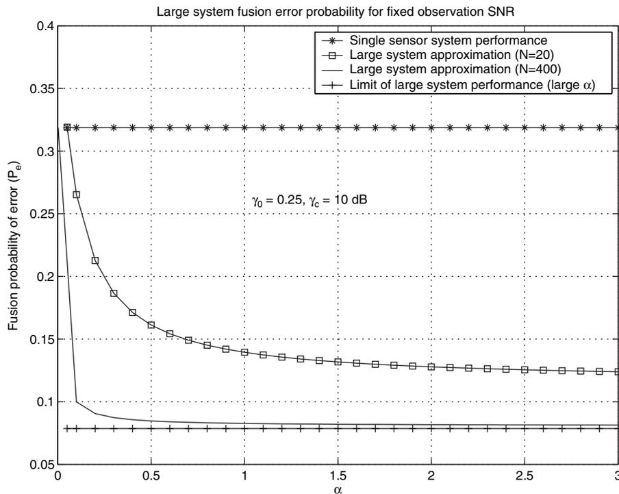
**Figure 6.4** Limit of Large Sensor System Approximation to the Fusion Performance in a Noisy, Bandlimited Channel Subjected to a Total Power Constraint when  $\alpha \rightarrow \infty$
