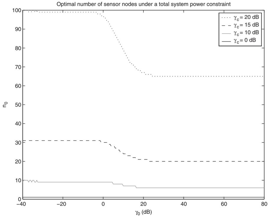
**Figure 6.7** Optimal Number of Sensor Nodes as a Function of the Observation SNR for a Given Channel SNR. The System is Under a Global System Power Constraint with Orthogonal Sensor-to-Fusion Center Communication
