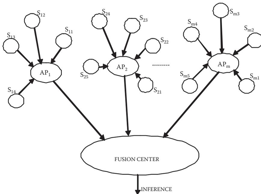
Figure 6.2 Sensor Network Topology
