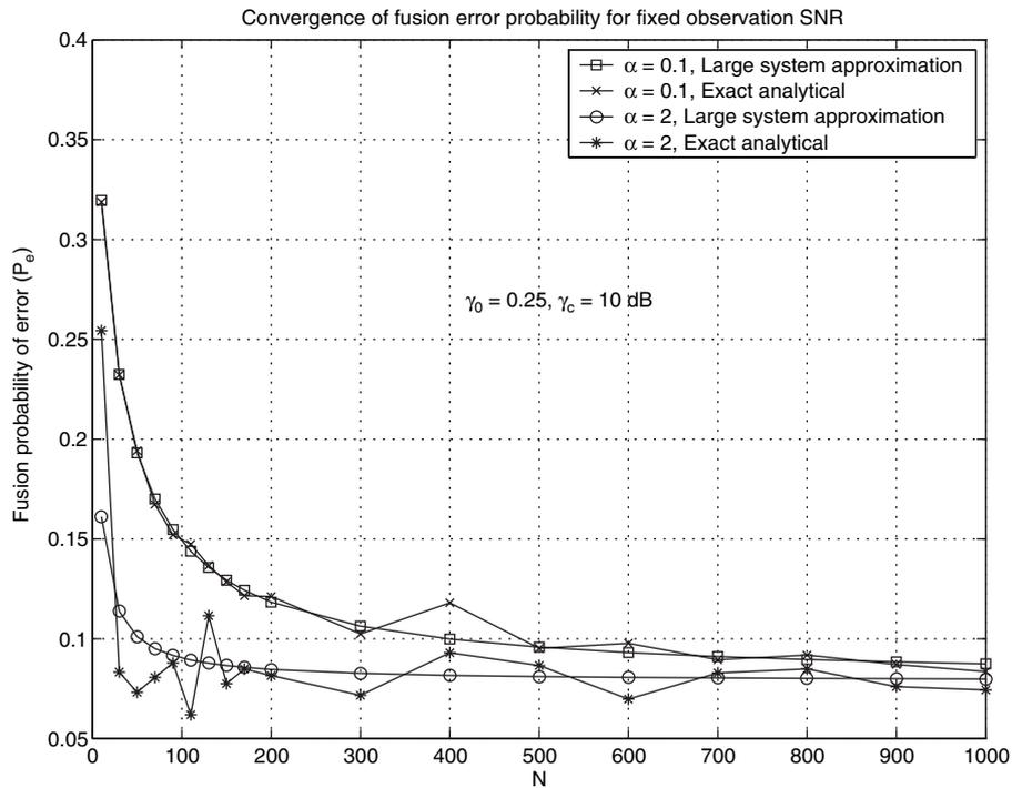
**Figure 6.3 Large Sensor System Fusion Performance in a Noisy, Bandlimited Channel Subjected to a Total Power Constraint**
