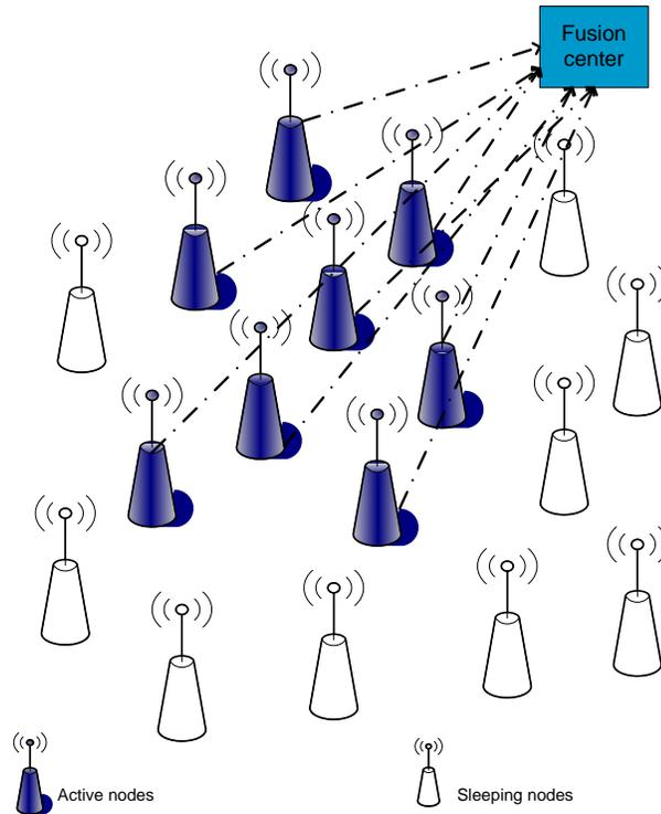
Figure 2.2: Centralized data/decision fusion architecture with a fusion center
