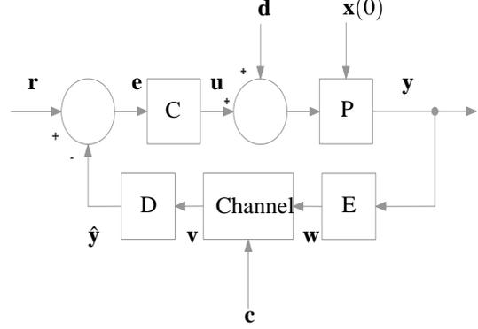
Fig. 7 Closed-loop system with additive disturbance.
