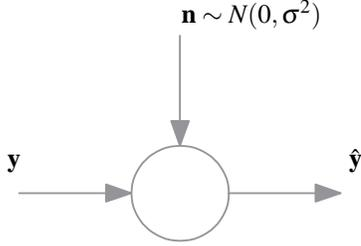
Fig. 5 AWGN channel scheme.
