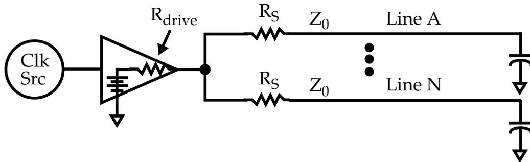
18) (5 pts) It is sometimes necessary to retard or advance the clock in one part of the circuit with respect to another, for example, as a means of reducing clock skew. Name (do not explain) three ways of adding a *fixed* or *adjustable* delay. Briefly explain how the following circuit allows delay to be adjusted.
