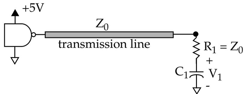
11) (5 pts) In order to eliminate reflections in end-terminated systems, the terminating resistor must precisely match the transmission line impedance. Name the sources for mis-match in end-terminated systems.
