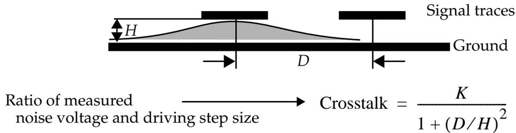
2) (5 pts) In our discussions over power/GND layout design, we indicated that the following scheme could be used in a two layer board, but would not work well for high speed logic. Briefly explain why this is true. Draw the return current path for the driver shown in the figure.
