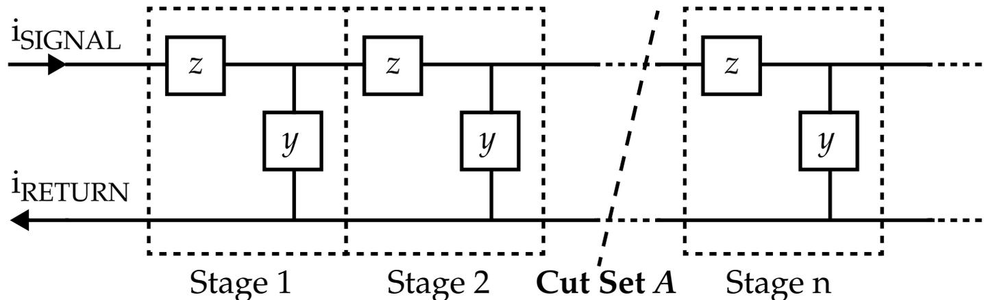
Impedance  $z$  consists of the series resistance of the signal and return conductors and inductance.
