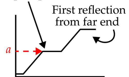
Here, the rise and fall times of the measurement setup complete well before one round-trip delay of the transmission line.
