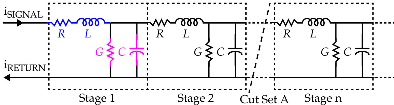
The series impedance  $z$  ( $R$  and  $L$ ) and shunt admittance  $y$  ( $G$  and  $C$ ) are *per unit length* of the transmission line (1 meter in our case).
