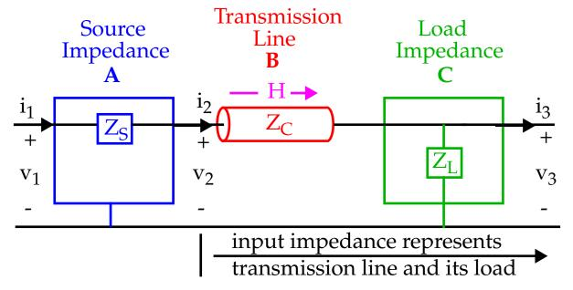
The input impedance of the loaded transmission line is obtained from the cascaded combination of BC
