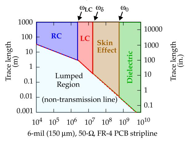
In lumped region, transmission line is short enough that it acts as a simple lumped circuit element.
