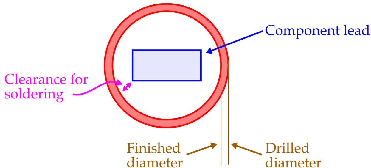
Holes are drilled with a *hole diameter tolerance*, e.g.,  $0.032 \pm 0.003$  in.
