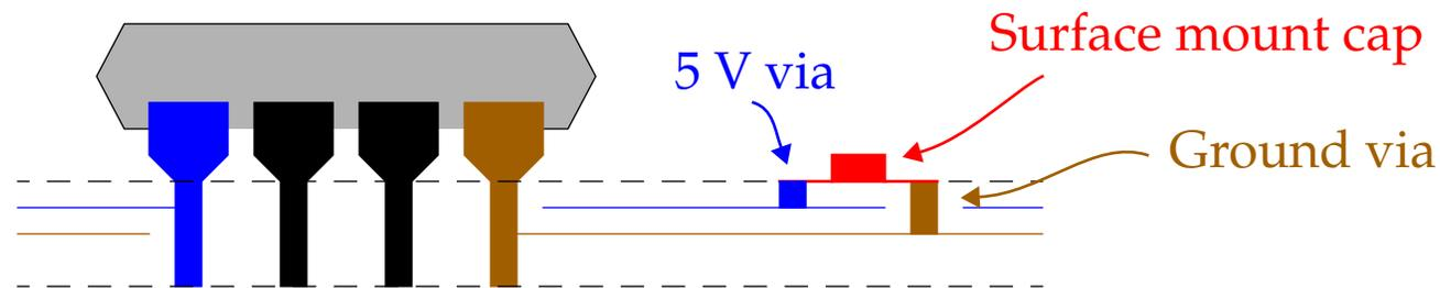
The vias used to connect the power and gnd planes to the bypass cap have a measurable inductance approximated by.
