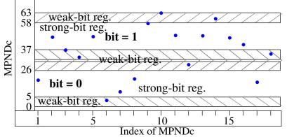
For example, if we were to re-collect the MPNDc's under other environmental conditions, i.e., with different supply voltage values and/or temperature conditions, the values will *shift* as shown by the following set of curves. The red dots represent a 'worst-case' shift that occurs to each MPNDc. The vertical shift in MPNDc's that are close to the bit-flip lines can result in the MPNDc value being re-classified from a '1' to a '0' or vise versa (identify where this occurs in the graph).
