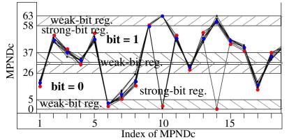
Therefore, MPNDc's that fall within the *weak-bit regions* are to be skipped when generating the bitstring. For example, the *strong* bitstring generated by processing the MPNDc's shown the graph is as follows:
