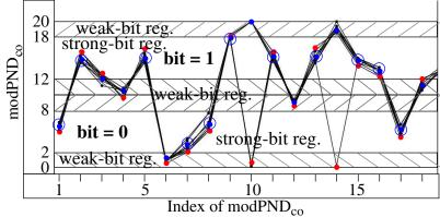
Therefore, modPND<sub>co</sub> that fall within the *weak-bit regions* are to be skipped when generating the bitstring. For example, the *strong* bitstring (SBS) generated by processing the modPND<sub>co</sub> shown by this graph is as follows (NOTE: values that fall ON the line are considered weak):
