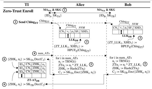
The AT are created by running the PUF in long-lived key (LLK) generation mode. LLK mode refers to the ability of the SiRF PUF to generate (enrollment) and then re-generate (regeneration) the same key later in time using helper data generated during enrollment.
