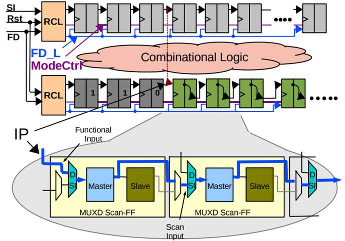
Fig. 1: REBEL embedded test structure.
