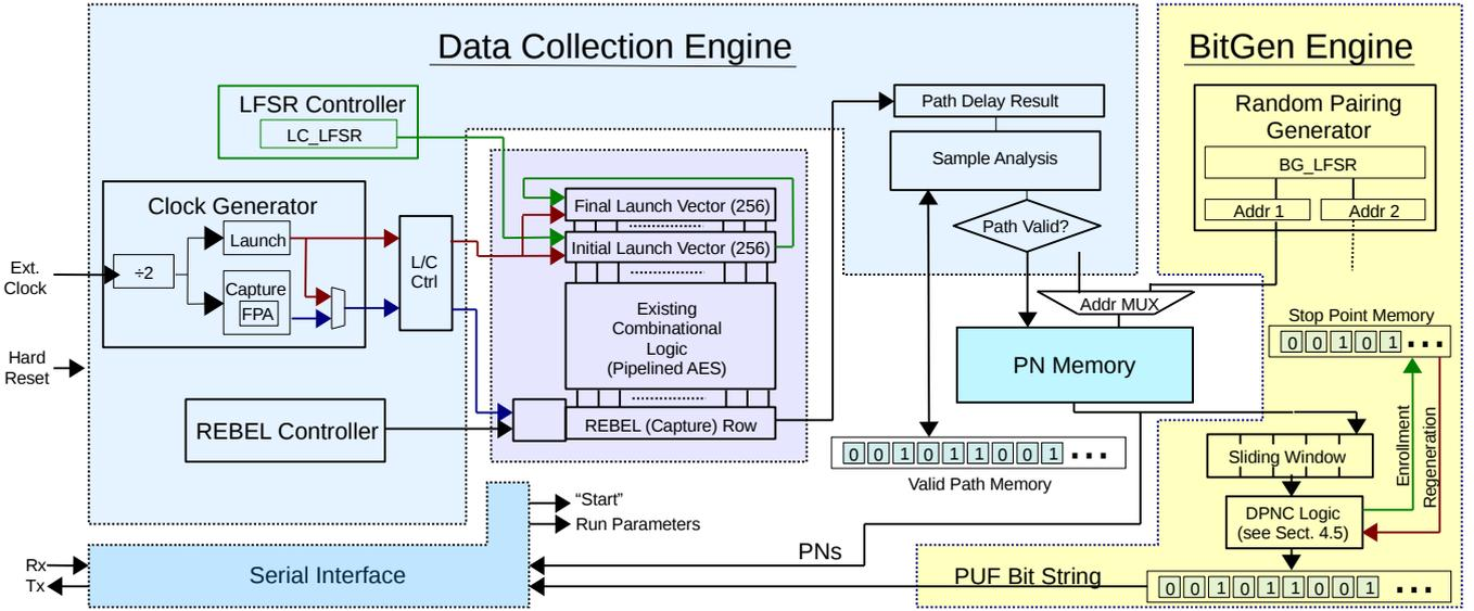
Fig. 2: Top-Level HELP System Diagram
