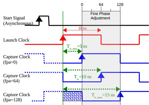
Fig. 3: Launch/Capture Timing Diagram
