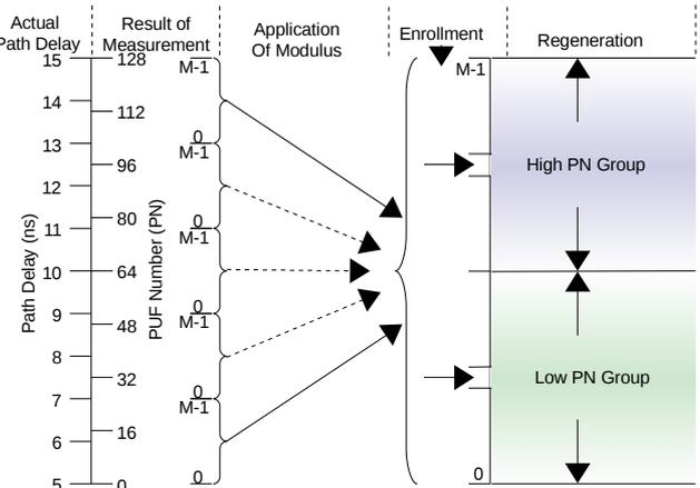
Fig. 4: Dual-PN Path Delay Binning Technique
