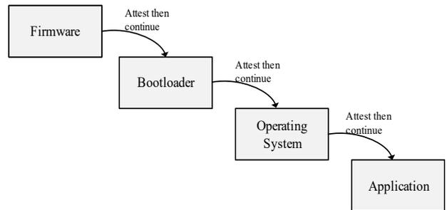
Figure 1. Secure Boot Software Chain of Trust
