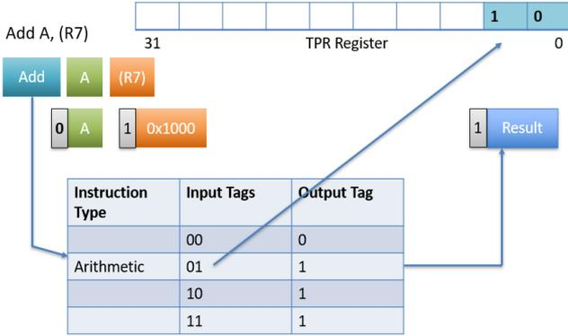
Figure 5. Tag Propagation Flow
