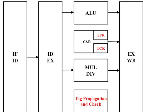
Figure 4. Modified execution stage of the processor pipeline
