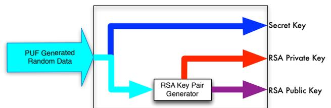
Fig. 3: Key generation method in ECE.
