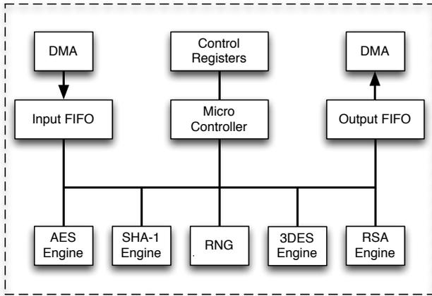
Fig. 1: Generic cryptographic unit.
