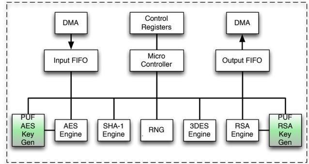
Fig. 2: Enhanced Cryptographic Engine.
