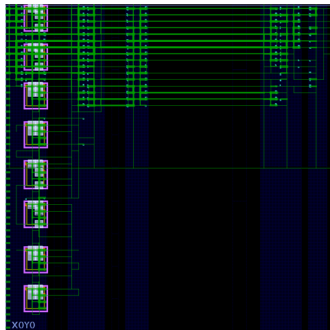
Fig. 3 Vivado implementation view showing layout of the SR-PUF hard macros.
