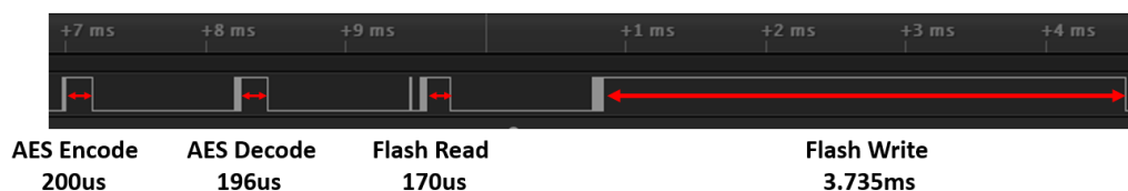
Figure 7. Timing characterization for Advanced Encryption Standard (AES) and flash read and writes.
