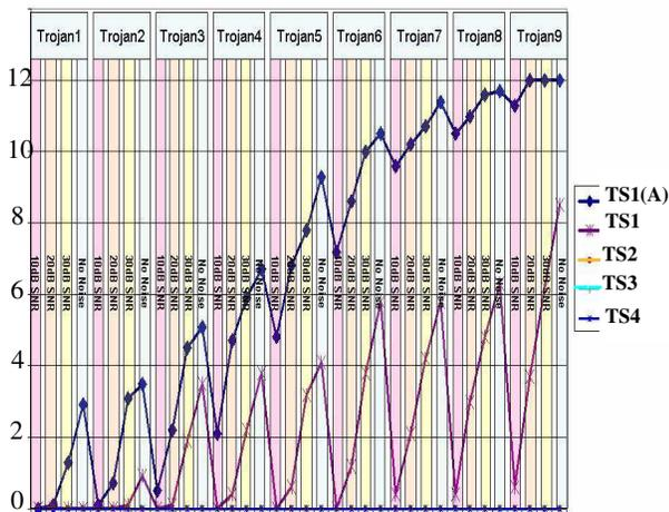
Figure 7. Number of Detections for TS1\_Active, TS1\_Passive (the original Passive stimulus), and the variants TS2, TS3 and TS4 that add random undesired switching activity to the circuit.
