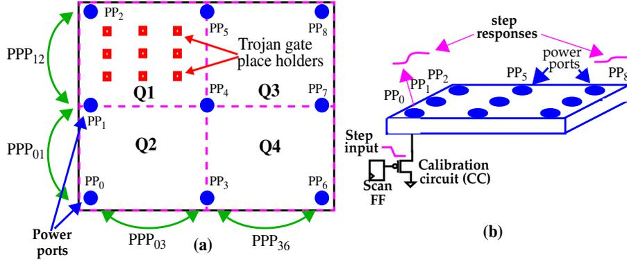
**Figure 1. (a) Architecture of the simulation model, each of the quads (Q1-Q4) contains a copy of C499 benchmark, (b) calibration circuit (CC) and step**
