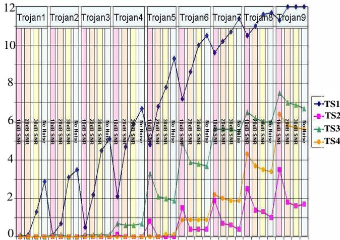
Figure 6. Number of Detections for TS1, the original Active stimulus, and for the three variants TS2, TS3 and TS4 that add random background switching activity to the circuit.
