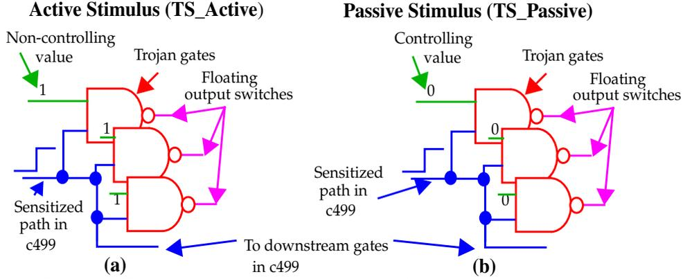
Figure 3. Trojan gate sensitization criteria under the two test sequences [4].
