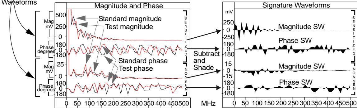
**Figure 2. Frequency Domain Signature Waveform creation procedure.**
