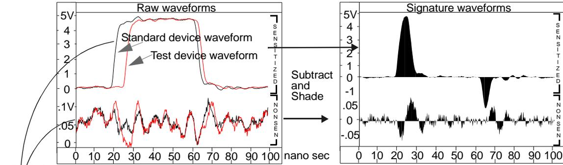
**Figure 1. Time Domain Signature Waveform creation procedure.**
