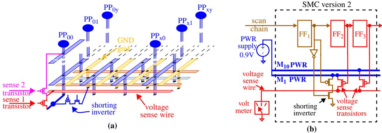
Figure 4. (a) Connections of a modified version of SMC (b) details of the modified SMC.
