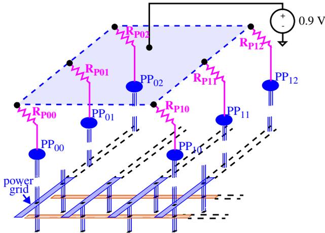
Figure 1. Power Grid Architecture
