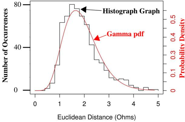
Figure 8. Gamma function fit of chip equivalent resistance histogram.
