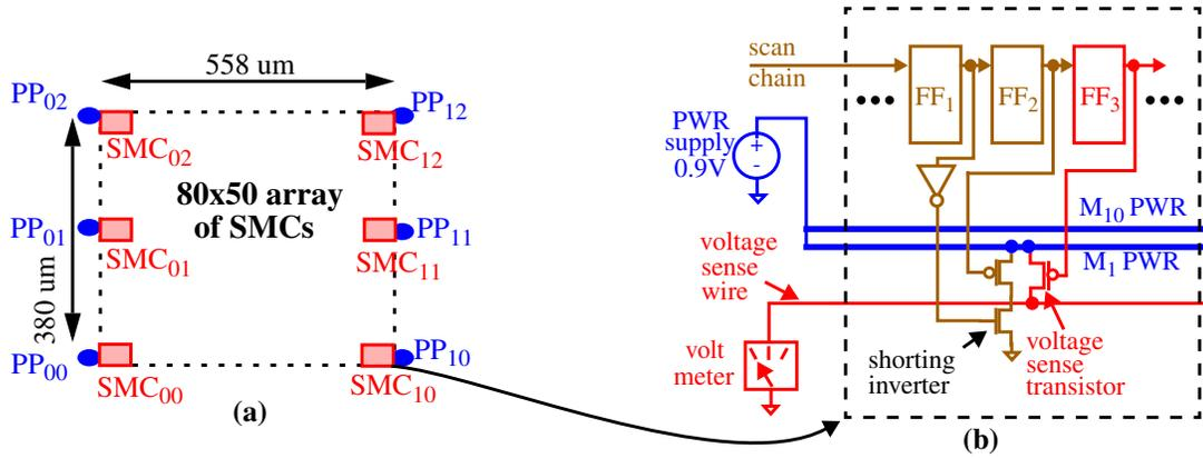
Figure 3. (a) Block diagram of the test structure and (b) details of the Stimulus/Measure Circuit (SMC).
