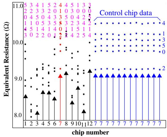
Figure 7. Equivalent resistance signatures for 12 chips and 12 control samples.
