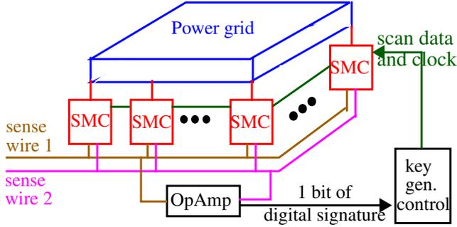
Figure 5. On-chip instrumentation for signature generation.
