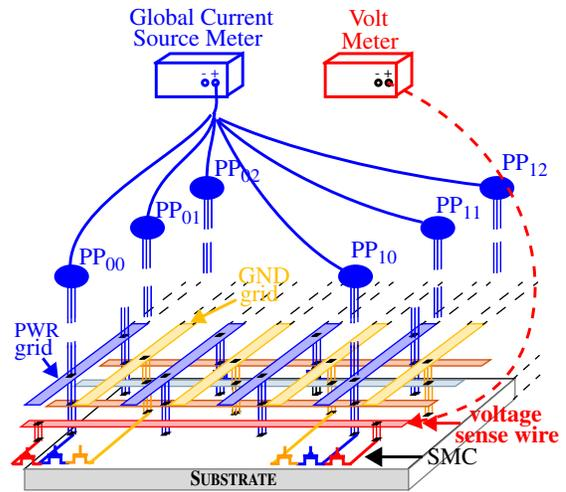
Figure 2. Instrumentation Setup
