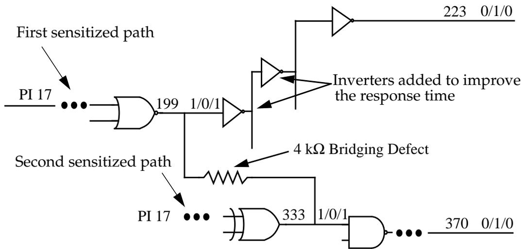
**Figure 1. Portion of the ISCAS85 c432 benchmark schematic showing a bridging defect.**
