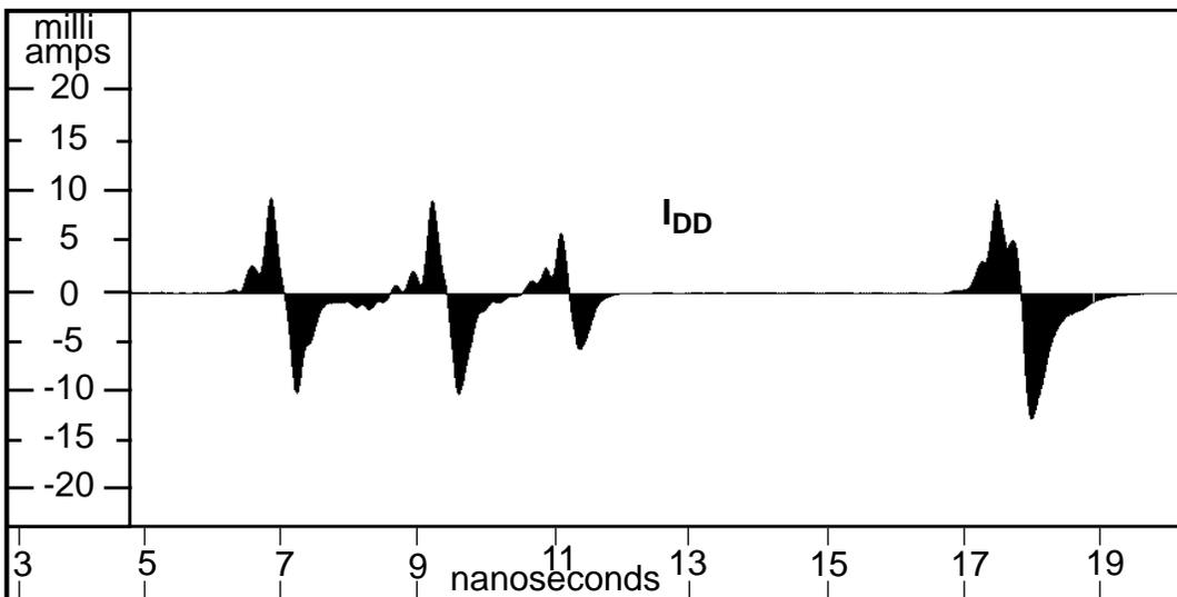
Figure 3. Current SW of the c432's supply rail in the presence of the bridging defect.
