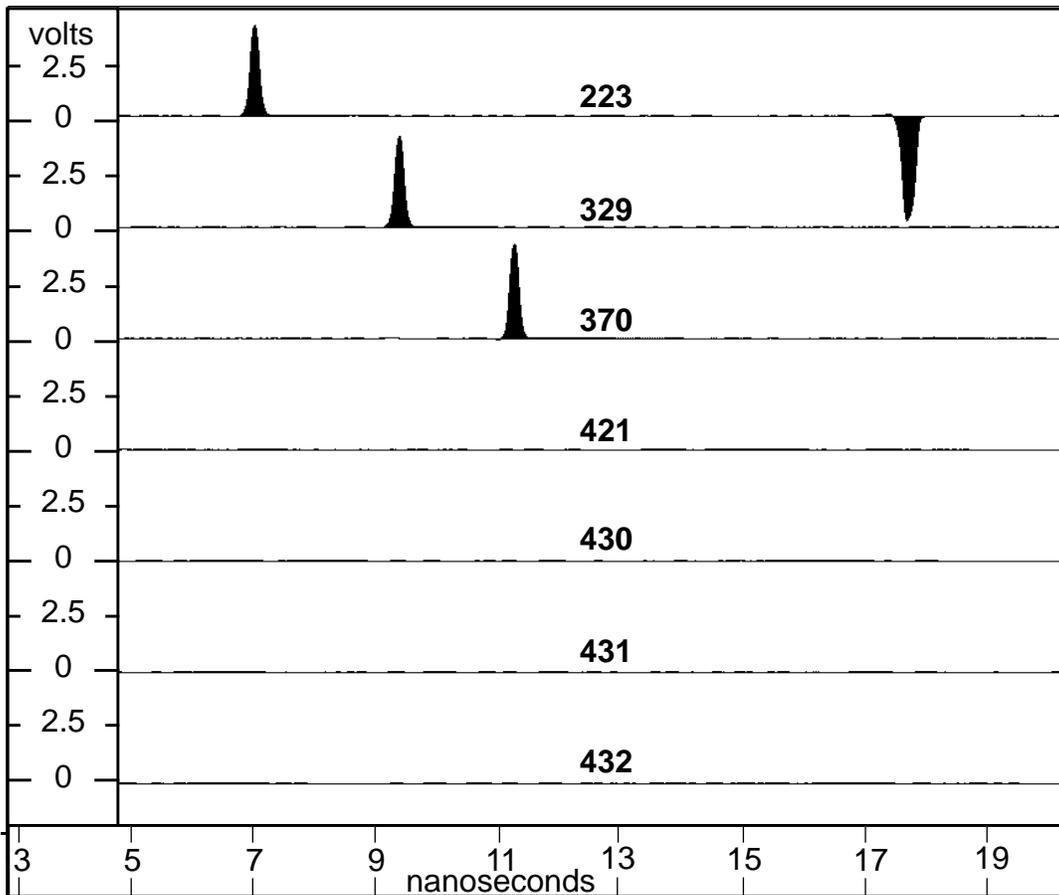
Figure 2. Voltage SWs of the c432's seven POs in the presence of the bridging defect.
