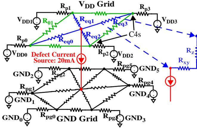
Figure 5. Equivalent resistance model of the Quad.
