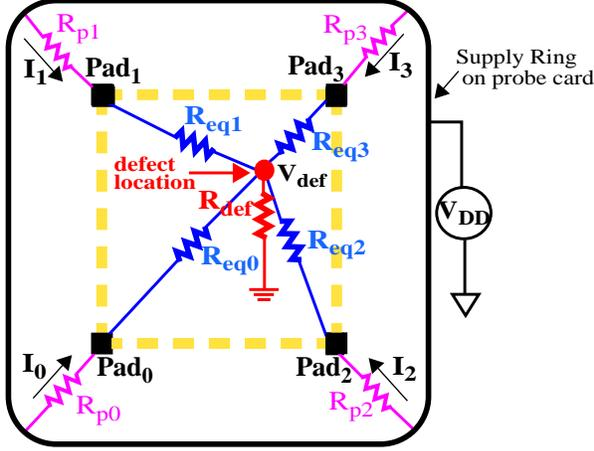
**Figure 1. Equivalent resistance model of the power grid with a shorting defect.**
