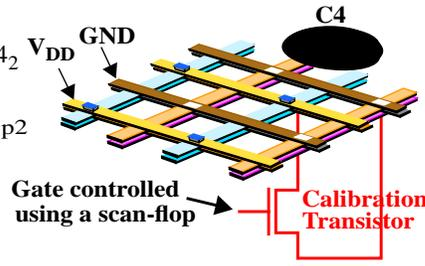
**Figure 14. Calibration Transistor and controlling scan-chain FF.**
