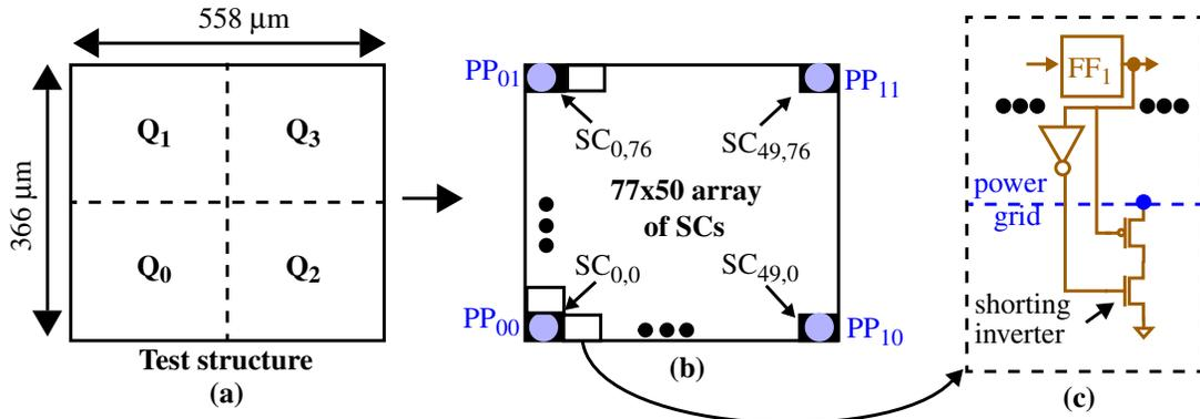
Figure 1: (a), (b) Block diagrams of the test structure and (c) details of stimulus circuit (SC).
