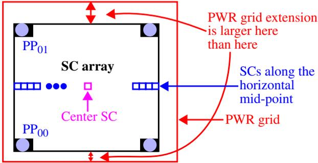
Figure 5: Actual power (PWR) grid architecture in the test chips.
