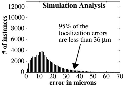
Figure 18: Localization errors using y-offset and curvature parameters derived from simulations.
