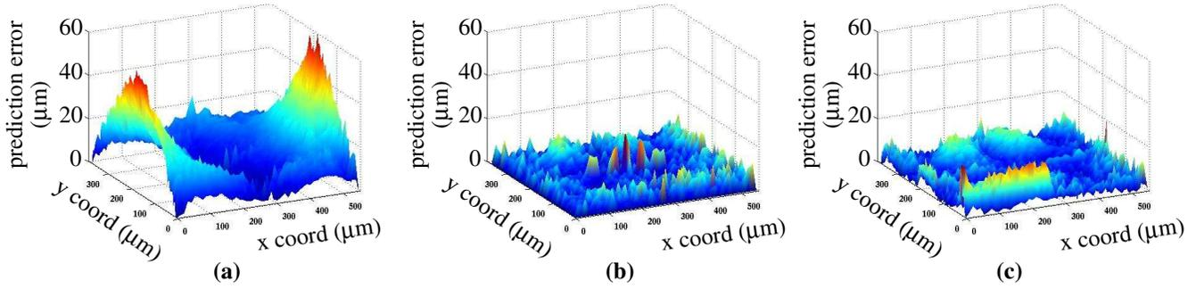
Figure 17: Localization errors for Chip C1 using a) simulation data, b) hardware data and c) ‘scaled’ simulation data.
