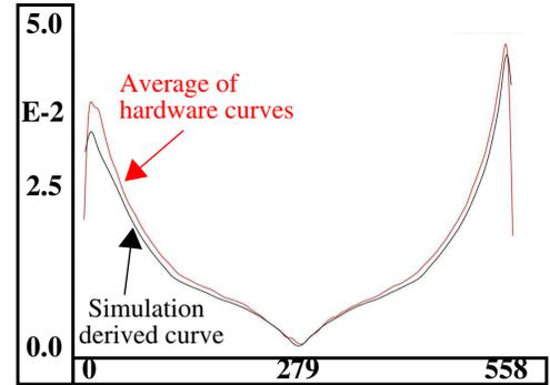
Figure 14: Hardware and simulation derived curvature parameter for  $PP_{00}$ - $PP_{10}$  pairing.
