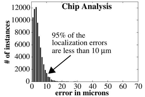
Figure 19: Localization errors using y-offset and curvature parameters derived from each chip.
