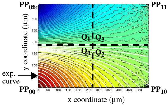
Figure 15: Chip C1 current fraction contours for PP<sub>00</sub>-PP<sub>01</sub>.
