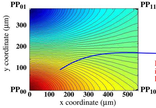
Figure 9: Current fractions contour curves,  $cf_{00_01}$ , from Fig. 7.
