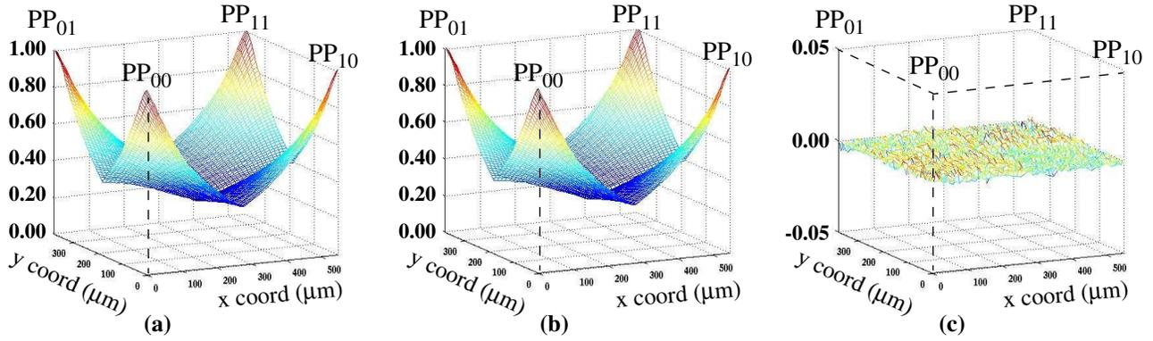
Figure 4: Calibrated normalized branch currents for Chip #1 (a) and Chip #2 (b) and their differences (c).
