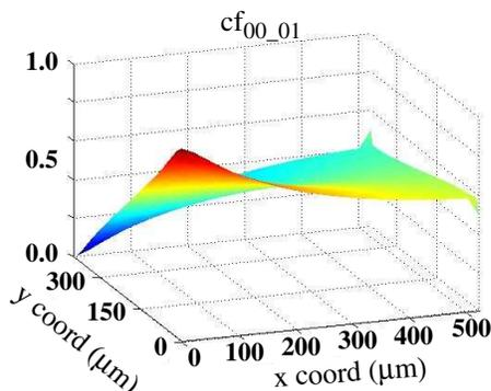
Figure 7: Current fractions,  $cf_{00\_01}$ , for 10 layer PWR grid model of chips.
