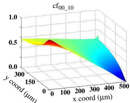
Figure 8: Current fractions,  $cf_{00\_10}$ , for 10 layer PWR grid model of chips.
