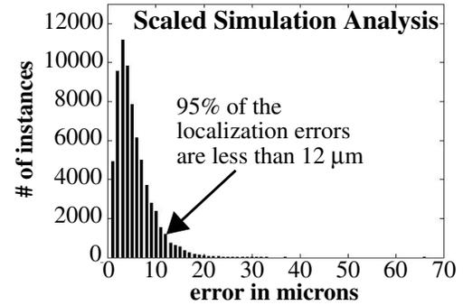
Figure 20: Localization errors using y-offset and curvature parameters from scaling the simulation curves.
