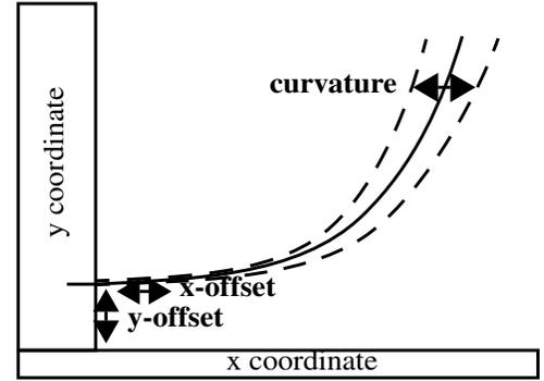
Figure 11: Exponential Curve and Parameters.
