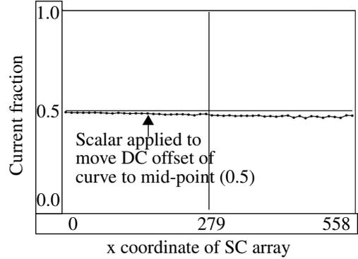
Figure 6: Distortion in the current distribution to PPs introduced by PWR grid architecture.
