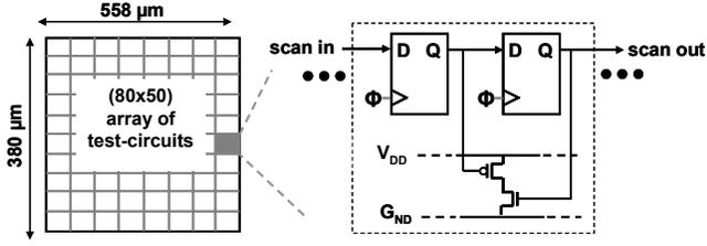
**Fig 1: Block diagram of the test macro and schematic of one test circuit element**
