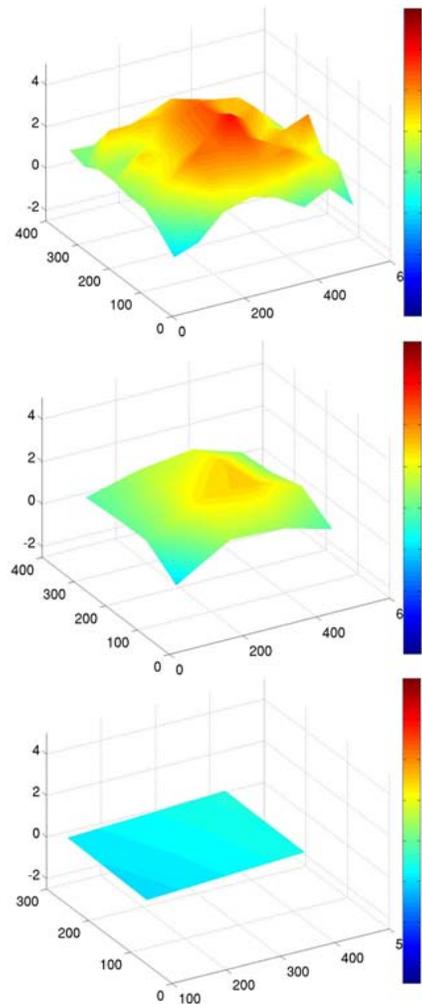
**Fig 8: Measured within-die spatial on-current profile with sleep island granularity of 64, 16, and, 4 islands (top to bottom).**
