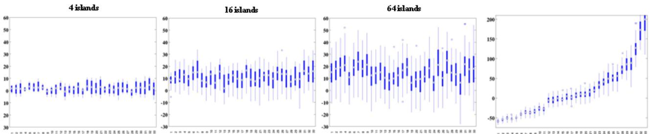
Fig 5: Measured within- die variation with 4, 16, and, 64 sleep islands for 33 chips. The range of variation increases with higher spatial granularity of islands.
