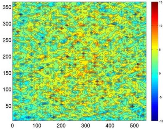
**Fig 7: Measured within-die on-current variation. All 4000 TCs are measured individually with only one TC active at a time.**
