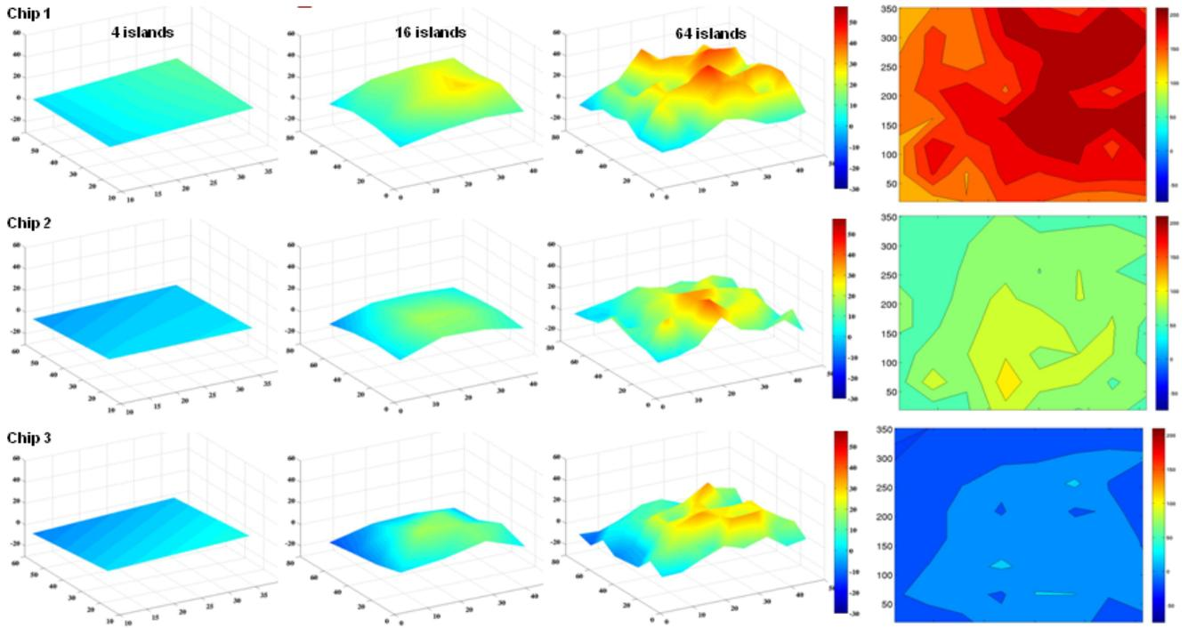
Fig 3: Measured within-die spatial leakage profile for three chips (top to bottom) with sleep island granularity of 4, 16, and, 64 islands (left to right)
