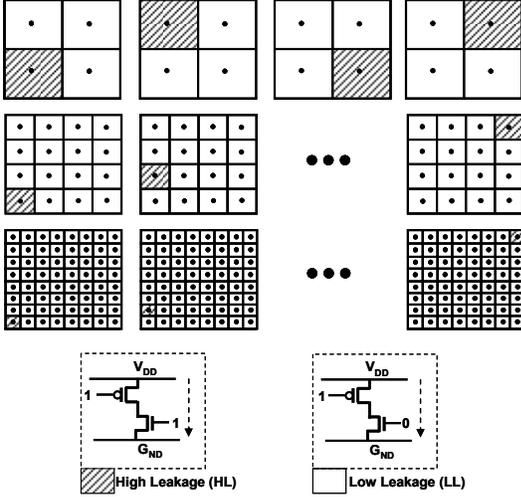
**Fig 2: Spatial leakage patterns created by putting test circuits in different spatial islands of the array in high leakage state. Three cases with spatial granularity of 4, 16, and 64 partitions are considered.**
