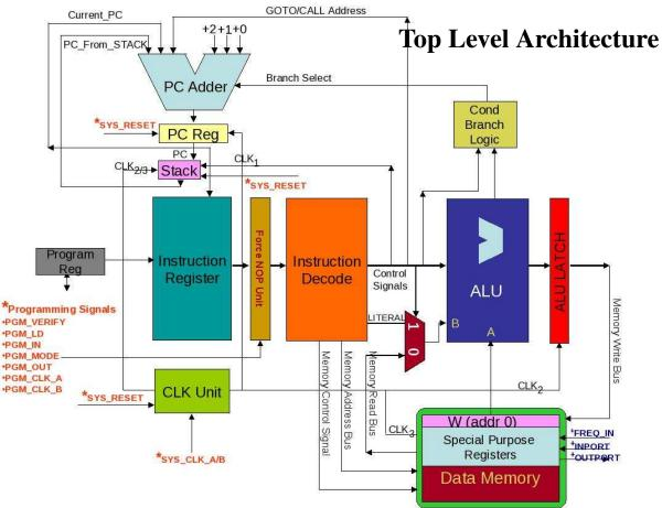
Red: external signals to control programming the microcontroller Blue: external signals for runtime communication/operation
