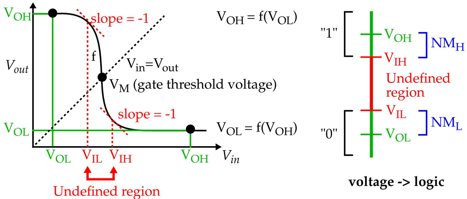
Even when an ideal input signal is applied to the input, the output often deviates from the ideal, due to noise and output loading.
