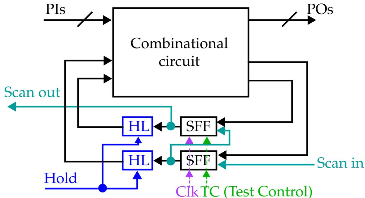
Each vector consists of two parts, bits for the PIs and bits for the state variables (SFFs).
