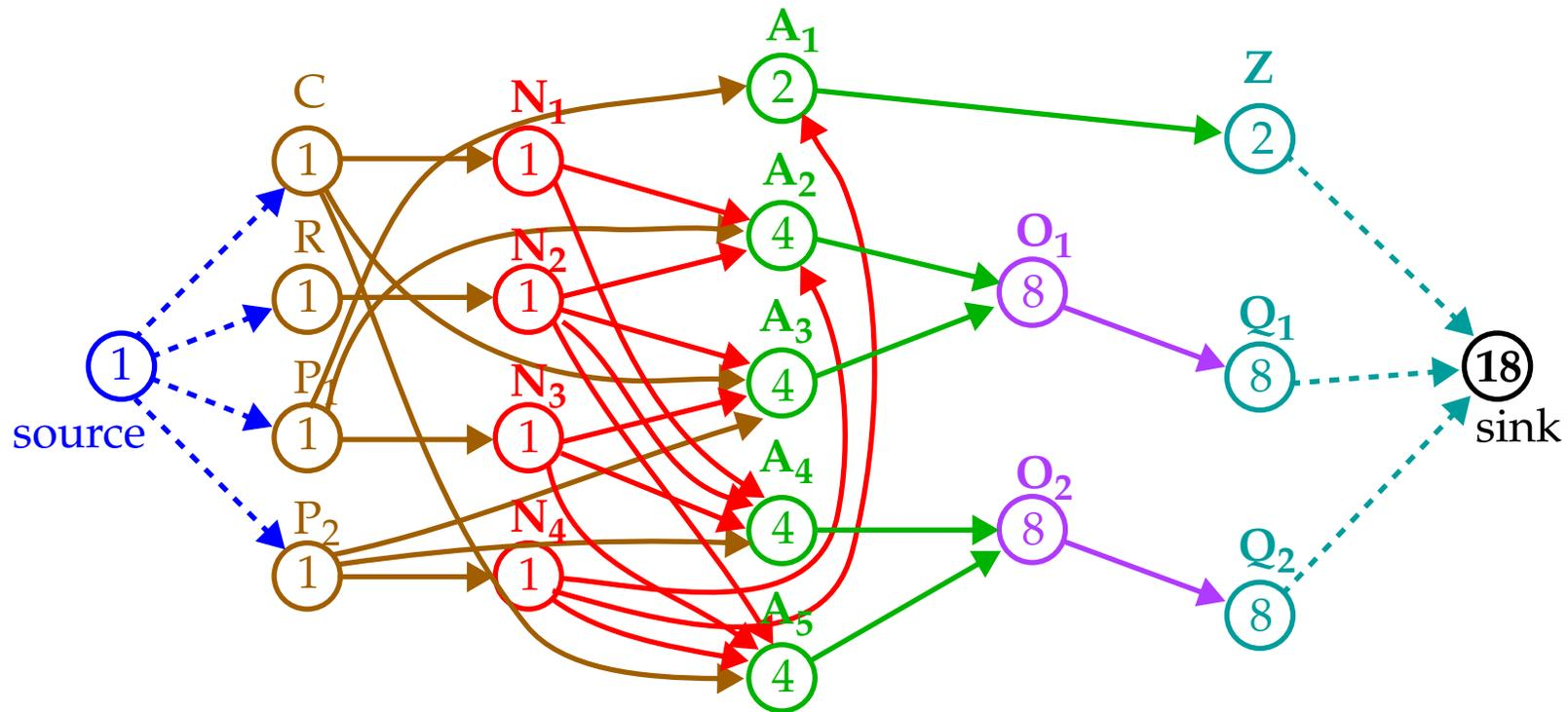
Vertices represent the PIs, POs and gates, edges represent signal flow.
