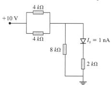
**1-35.**  $I_s = 2\mu A$  for the diode. Calculate  $V_D$  and  $I_D$ .
