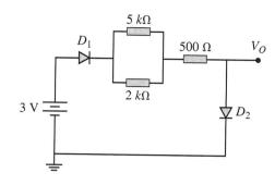
**1-32.** Calculate the voltage across the diodes given that the reverse bias saturation current in  $D_1$  is  $I_{s1} = 175$  nA, and  $I_{s2} = 100$  nA.
