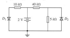
1-34. Calculate the diode current and voltage.
