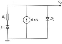
**1-31.** Diode  $D_1$  has a reverse bias saturation current of  $I_{s1} = 1$  nA, and diode  $D_2$  has  $I_{s2} = 4$  nA. At room temperature, what is  $V_O$ ?
