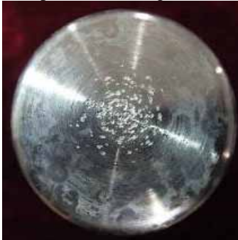
Figure 6. The photo of the surface of the coaxial extractor after the experiment.
