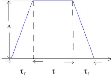
Fig. 1 Trapezoidal pulse as used in bioelectric experiments
