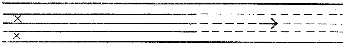
Figure 2 Two-element series Blumlein generator with output line.
