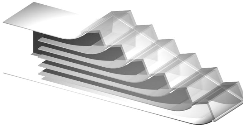
**c. Three-dimensional view of a split waveguide.**
