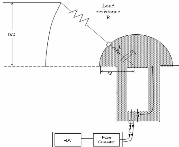
Figure 4. An oscillator that switches into an antenna.
