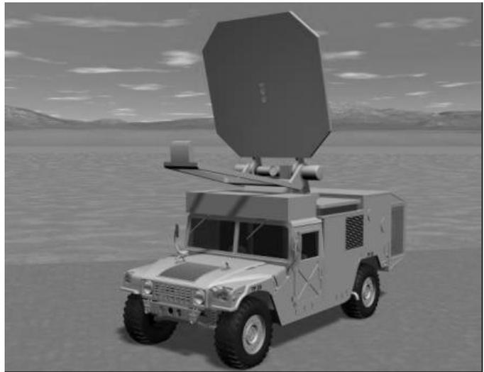
**Figure 9. The Vehicle-Mounted Active Denial System Concept**
