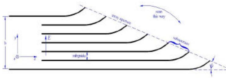
**b. Side view of a split-waveguide.**
