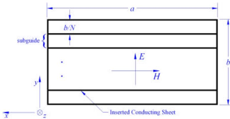
**a. Cross section of a split-waveguide.**
