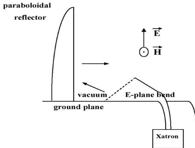
Figure 2. Half-reflector Phaser.
